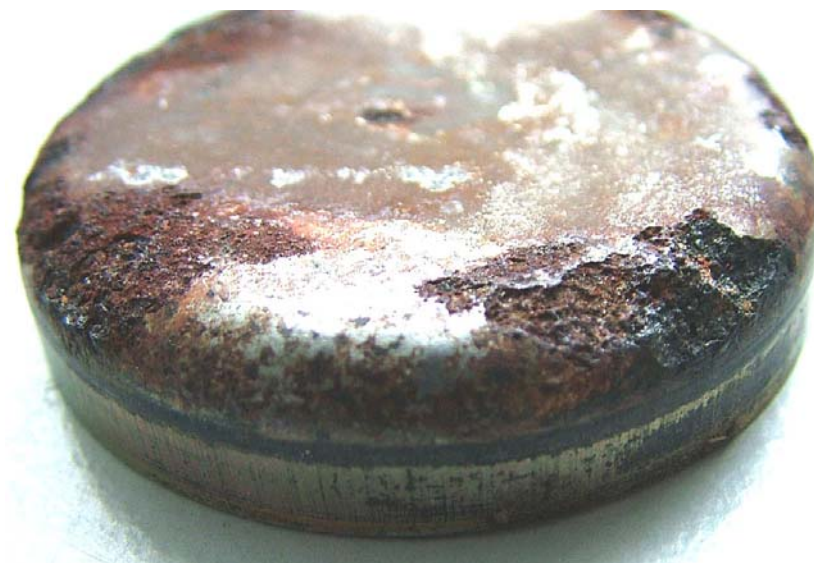
A 6 Sealing cover, corroded
