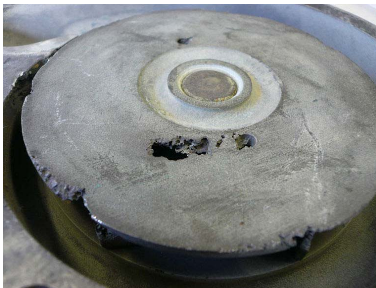
A 10 Flywheel of the coolant pump, cavitated
