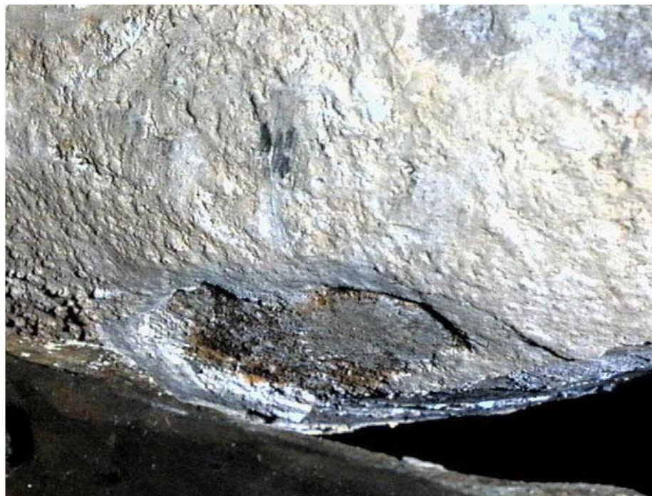
A 8 Limescale deposits on a cylinder liner
