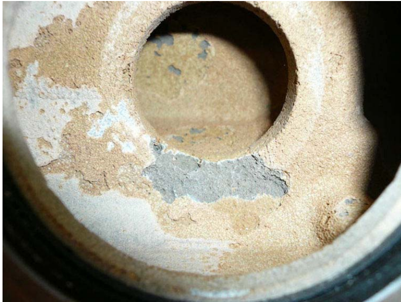
A 7 Aluminium thermostat cover, corroded
